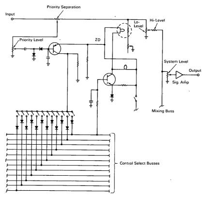
A problem generally exists when using several microphones fed into a common system. Sound originating at any given signal source and picked up by multiple microphones, provides an effect similar to multiple sources picked up by a single microphone. This effect results in poor articulation (speech clarity) at the output (speaker) because of the varying phase shift at different frequencies and distances.
