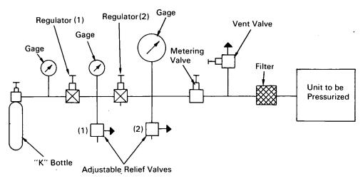
Note: Schematic Shows Assembly for Low-Pressure Range (0–60 psig). Relief Valve (1) and Regulator (2) are Omitted for High Pressures (60–2000 psig)
