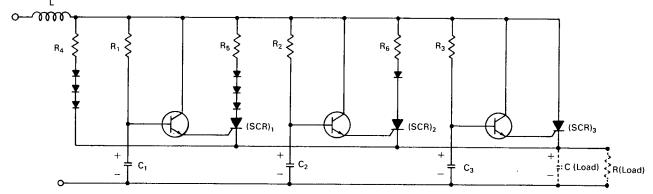
This circuit limits the turn-on current transient to a specified amplitude and provides a low-impedance path between supply voltage and load after a prescribed time interval. The circuit offers a wide range of flexibility in adjusting peak current and time to complete connection to the load. It is more compact and lighter than a comparable limiter circuit which uses a large choke but which is still not effective where large load capacities are involved.
