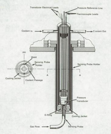
A compact water-cooled mount for miniature pressure transducers, which has been developed, permits locating the transducers in hotter and more confined environments than was previously possible. Compactness was attained by utilizing pressure transducers ½ inch in diameter by ¼ inch in length, with connecting leads and reference pressure tube extending from the rear. Good response at frequencies to several hun-
