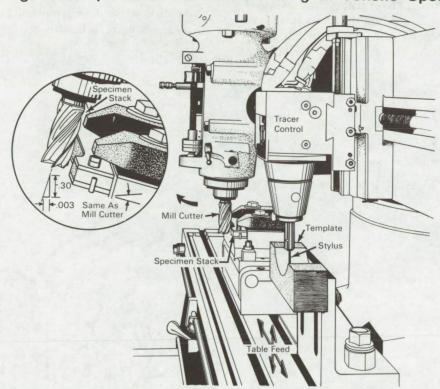
Machining Technique Prevents Undercutting in Tensile Specimens
