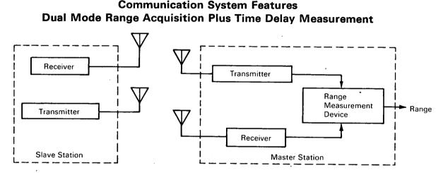
A communication system has been designed to overcome two very troublesome problems involved in following and measuring the movements of high velocity airborne or space probing vehicles.
