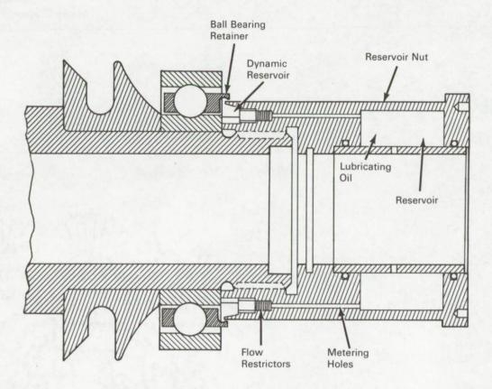
A device has been designed to satisfy a need for a means of supplying controlled amounts of lubricating oil to ball bearings only during operation of the bearings. The main purpose of the device is to ensure optimum supply of lubricant to increase the operating life of the bearing without application of additional power. Wick feeds are not satisfactory because they
