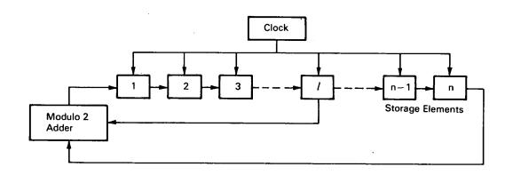
Pseudonoise digital modulation is used in a number of tracking and communications systems. In most cases it is necessary that the receivers of such systems bring an identical locally generated pseudonoise signal into time synchronism with the incoming pseudonoise signal. This acquisition process may require a relatively long time because of the period of the pseudonoise signals used and because of the autocorrelation properties of the signals.
