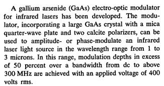
The large single crystals of gallium arsenide used in the modulators were grown by the horizontal Bridgeman technique. They have uniformly high resistivities (exceeding 10<sup>6</sup> ohm cm), are strain-free, and are comparable in quality to that of good optical glass. The small size and poor electrical and optical quality of most electro-optical crystals previously available have limited their usefulness as laser modulators.
