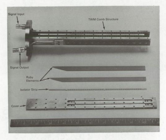
A traveling wave maser (TWM) that operates at S-band frequencies is characterized by a greatly improved gain-bandwidth product with relatively low equivalent-noise temperature. Tests indicate that its performance exceeds that of any other type of S-band amplifier. The improved performance and easier fabrication of the new maser were achieved by combining the best features of previous designs in a single struc-
