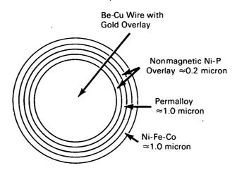
Advanced memory systems are needed in modern computer technology to keep abreast of constant improvements being made in electronic circuitry and packaging techniques. The plated wire memory in particular appears most attractive because of its high output compared to planar thin film memories and also because of its high speed and simplicity.
