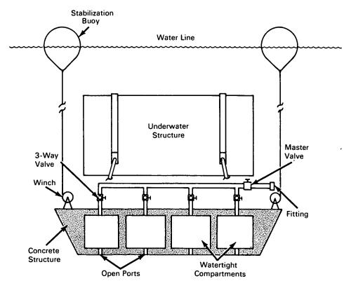
Underwater habitation experiments have shown that transportation of the structure, placing it in the water, transportation of the required ballast, and the placement of ballast on the structure at sea are difficult and expensive. The cost of lead ballast alone may exceed the cost of a habitable structure by a factor of two or more. A ballast barge concept should be relatively low cost, easily operated, and readily supported from small surface vessels.
