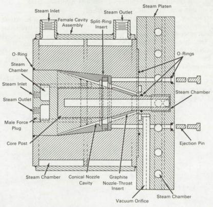
A single molding process has been developed to ensure that plastic parts (of a given mechanical design) produced from a conventional thermosetting molding compound will have a maximum tensile strength. The process, specially developed for molding an asbestos-phenolic rocket motor nozzle incorporating a molded-in-place graphite insert, can also be used for other thermosetting compounds to produce parts with improved physical properties.
