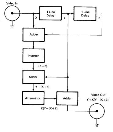
The circuit represented by the block diagram is designed to enhance vertical resolution in electron beam, raster scanning systems exhibiting aperture distortion in the vertical direction. A sensitized area (image) whose boundary lies more than one sweepwidth away from the scan beam position produces a video output when the scan beam nears it. This effect produces vertical elongation in the reconstructed images of all sensitized areas on the surface
