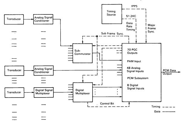
Three problems existed in earlier PCM subsystems, minimal data handling capability, fixed format, and system size, which could not always be tolerated. A PCM subsystem which is programmable, high speed, and small is required to support the variety of signals inherent to a sophisticated spacecraft, for example.
