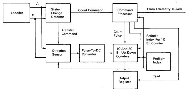
Accumulator for Shaft Encoder
