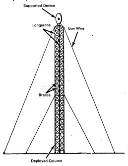
In many situations, it is required that certain equipment, such as instruments for measuring pressure, temperature, humidity, and the like, be raised to a level appreciably above that where data is to be recorded and evaluated. In cases of certain military applications or those requiring that short, discrete time increments be taken advantage of, a quick and dependable means of raising such instrumentation is needed.
