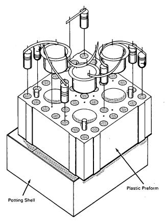
A reliable method has been developed to facilitate the fabrication of small lots (prototypes, experimental circuits, and other limited production quantities) of welded cordwood circuits. The essential feature of this method is the use of a molded plastic preform, or nesting jig, which retains the components during welding and electrical checkout. The preform also facilitates encapsulation of the welded module when used with a conventional potting shell. As the preform
