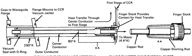
SIGNAL INPUT COAXIAL LINE ASSEMBLY
