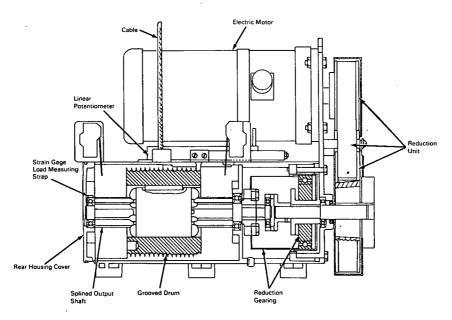
An improved control system power unit for driving the control surfaces of very large controllable parachutes has been designed. The improved design features (1) subassemblies simpler and less expensive for determining control surface position and cable loading and (2) protection of the load sensor against the possibility of damage during manipulation.
