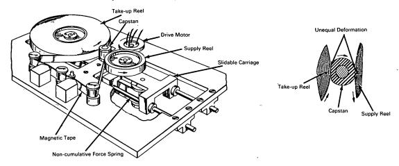
A magnetic tape recorder, which has been designed, is of simple, rugged construction and operates with relatively little power.
