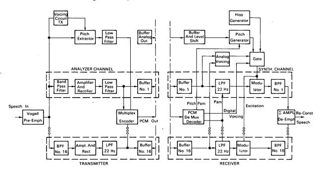
An existing, commercially available electronic voice encoder (Vocoder) has been modified to include an independent analog mode of operation in addition to the conventional digital mode. The Vocoder is a bandwidth compression equipment that permits voice transmission over channels having only a fraction of the bandwidth required for conventional telephone-quality speech transmission.
