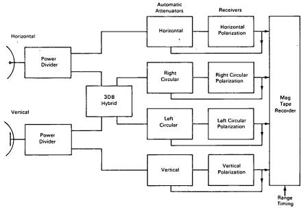
Accurate inflight signal-strength measurements are necessary to verify the design and performance of RF telemetry systems. Such measurements may also be used to analyze the effect of rocket exhaust flames on the phase and amplitude of signals. Other propagation anomalies may be revealed by accurate signal strength information.
