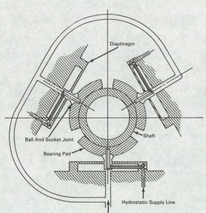
Pneumatic Line for Load Limiting
