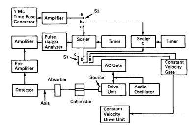
An instrument has been designed for the measurement of mechanical vibrations in transducers at amplitudes in the range of a few to 100 angstroms. Vibration measurements in this amplitude range cannot be accomplished by ordinary optical means. This instrument utilizes the Mossbauer effect, the phenomenon of the recoil-free emission and resonant absorption of nuclear gamma rays in solids, which was discovered by Rudolf L. Mossbauer in 1957.
