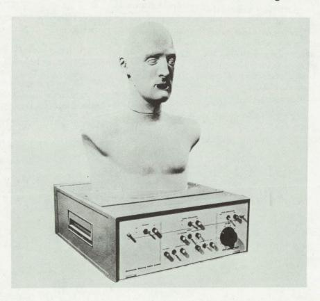
In order to conduct acoustical tests in a laboratory fashion, that is with variations and repeatability not dependent on human subjects, it was decided to design and fabricate an electronic dummy (ED). The ED was proposed as a manikin to represent the average male torso from the Xiphoid process upward and to include an exact acoustic replica of the human head.
