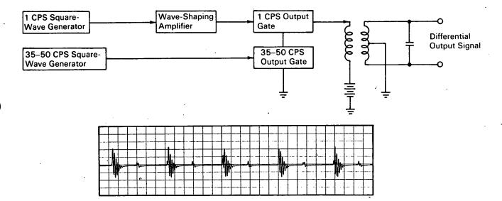
A phonocardiogram that produces a pattern of electrical signals exactly duplicating, in time and amplitude, the sounds of the human heart, has become a very important tool in physiological monitoring of astronauts in flight and during flight simulation. To calibrate and check out such a device, it is necessary to simulate, with accurate control, the timing and amplitude of heart activity signals.
