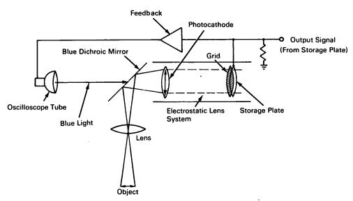
A particular design concept is presented for an unattended television photo-scan camera-tube where the complexity of internal beam scanning and critical beam-current adjustment of the conventional image orthicon is avoided by optical scan readout.
