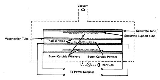
A vapor deposition method of growing boron carbide whiskers is described in Tech Brief 65-10262. Although the chimney-type furnace used in that method produced whiskers of generally high strength and in sufficient yield for tensile testing and characterization studies, the whiskers were short and had both a taper and a curvature.
