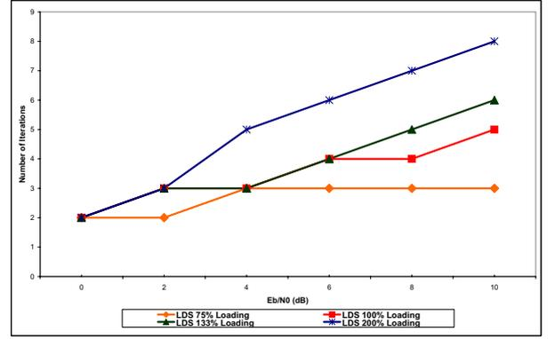
Fig. 3. Convergence Rate of Chip-Level Iterative Multiuser Decoding
