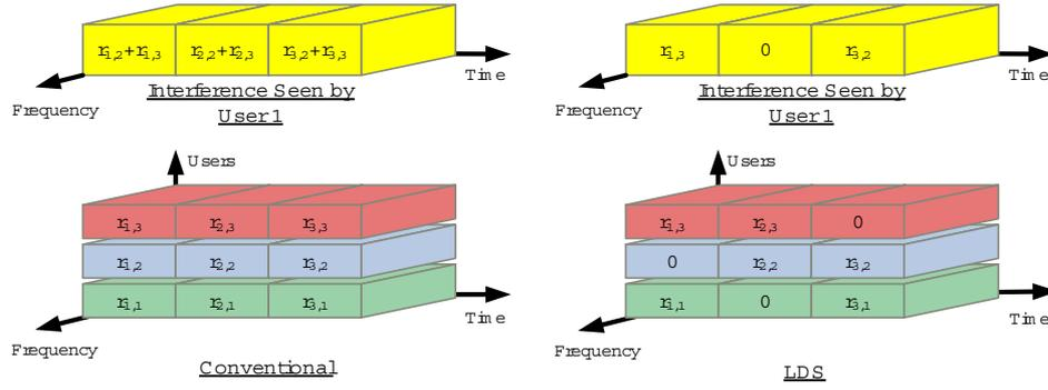
Fig. 1. Interference Seen Pattern of Conventional and LDS Structure of DS-CDMA Systems
