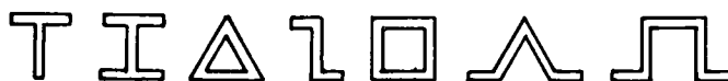
Cross sections of some typical stiffeners (extruded or formed from sheet metal clad with Al-Si braze alloy)
