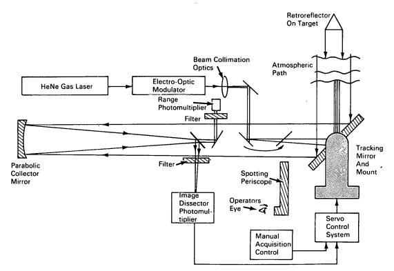
A precision laser tracker has been constructed and tested which is capable of tracking a low acceleration target to an accuracy of about 20 microradians rms. In tracking high acceleration targets the error is directly proportional to the angular acceleration. For an angular acceleration of 0.6 radian/second<sup>2</sup> the measured tracking error was about 0.1 milliradian.
