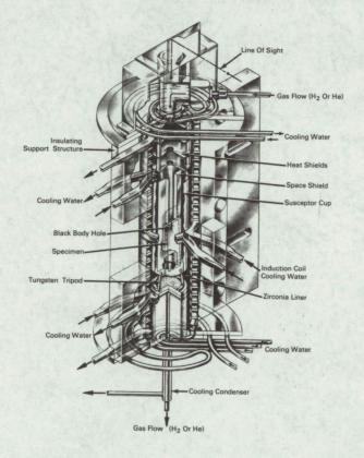
The problem: To construct a hydrogen (or inertgas, e.g., helium) atmosphere induction furnace that will operate at temperatures up to 5,350°F. The furnace must heat up and cool down rapidly during an effective life of several hundred cycles in normal use at operating temperatures below 5,000°F.
