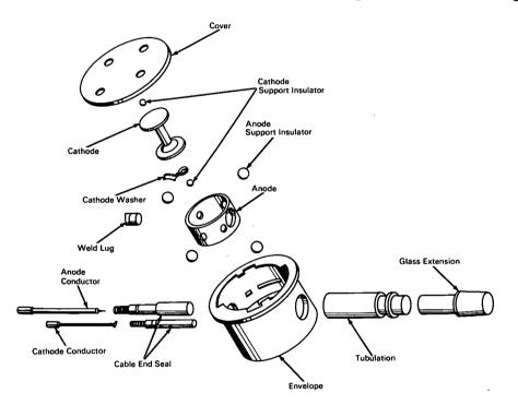
**The problem:** To design an ionization pressure gauge to accurately measure pressures to 10-14 torr. Hot filament gauges suffer from contamination by chemically active gases that change cathode emissive properties and hence gauge sensitivity. Cold cathode gauges of the glass envelope type suffer helium permeation of the envelope walls that reduces gauge sensitivity and requires frequent bakeout, thus losing its usefulness for long-period monitoring.
