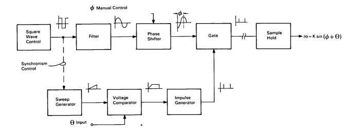
**The problem:** To provide an electrical signal whose magnitude is proportional to the trigonometric sine of a given angle  $\theta$ , plus or minus a fixed phase angle  $\phi$ , when  $\theta$  is linearly proportional to the magnitude of an input electrical signal. Prior methods have used rotating electromechanical components whose dynamic accuracy is limited by the slow response time of servo controls.
