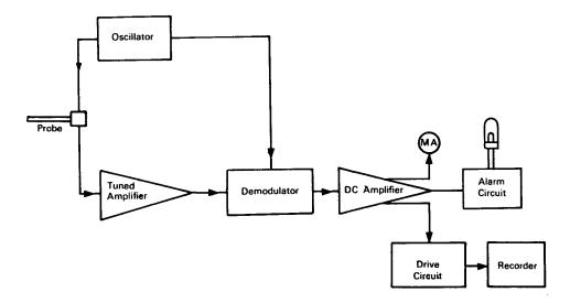
**The problem:** Detecting internal mechanical flaws or the presence of hard spot impurities in electrically conductive tubing or complex tubular structures.
