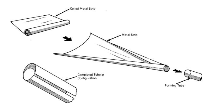
**The problem:** To devise a method of converting a strip of copper or copper-based alloy into a springy material that can be rolled into a compact coil which will spontaneously open to form a tube in the long direction of the strip when a restraining force is released. The strip must be capable of withstanding repeated cycling between the coiled and tubular forms.
