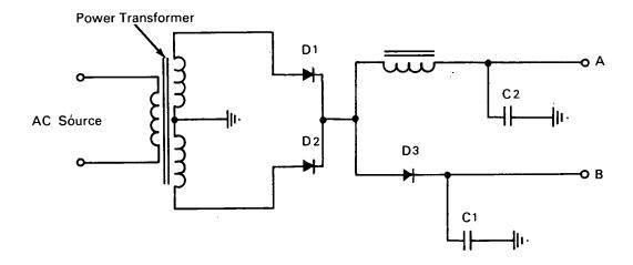
The problem: To design an efficient circuit that will provide two different dc output voltages from an ac source. Conventional circuits require either a precisely tapped transformer with a separate rectifier and filter for each voltage output, or dropping resistors, which waste power and result in poor regulation.
