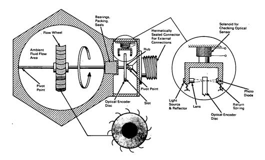
The problem: Accuracy in magnetic flowmeters is degraded by such things as ripple current, power input amplitude variations, and changes in duty cycle. A flowmeter is needed that operates independently of other system inputs.
