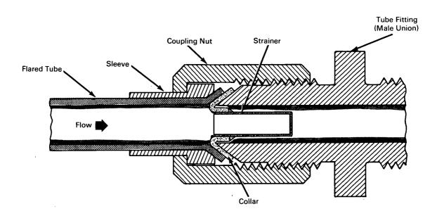
**The problem:** To provide a simple, easily replaceable strainer that can be readily installed in standard flared-tube fittings.
