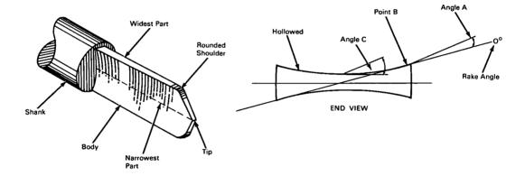
The problem: In drilling laminated materials, drill bits have operated by a scraping action due to their zeroto-negative radial rake angle. This has resulted in delamination due to tearing of the material at the ends of the holes and heat generated in bit and material.
