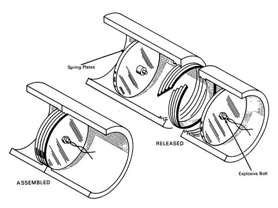
The problem: To quickly and cleanly separate two structural members by remote control. A design is needed that lends itself to various configurations and sizes of structures.
