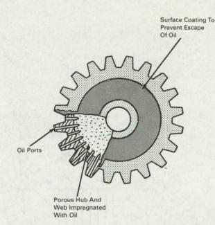
**The problem:** To provide a reliable automatic means for replenishing gear mechanism lubricants that can be expected to dissipate in the harsh environment of space or through extended operation in an atmospheric environment.
