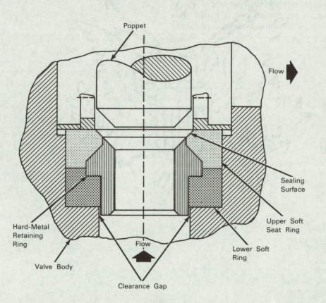
**The problem:** To design a soft-seat poppet valve that will provide positive closure against fluid without damage to the seating surface on repeated cycling. **The solution:** A poppet valve incorporating two compressible soft rings and a retaining ring of hard metal. Sealing is effected when the poppet seat is forced into intimate contact with a mating surface on one of the soft rings.
