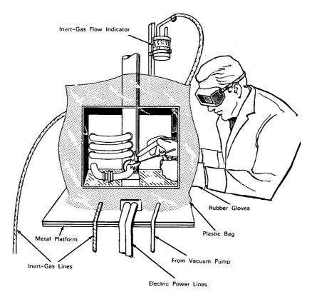
The problem: Available chambers in which a protective inert-gas atmosphere is maintained for welding and brazing of certain metals are relatively expensive and do not accommodate large workpieces, particularly when they are part of fixed equipment such as pipelines and manifolds.
