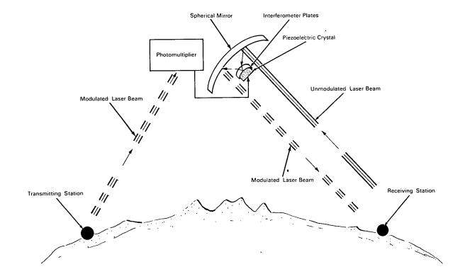
**The problem:** To develop a laser-beam system for communicating between two remote stations via satellite.
