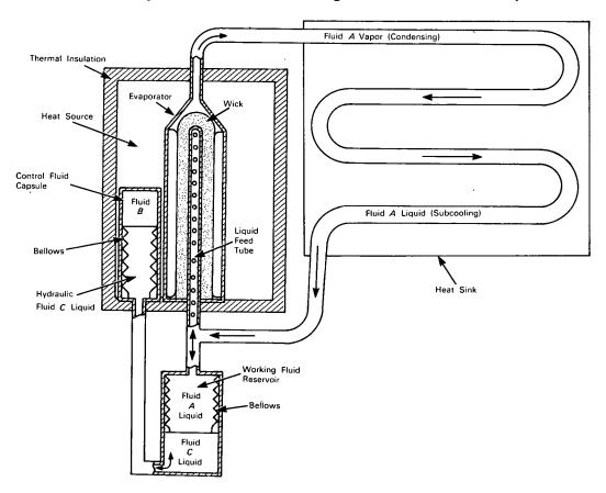
The problem: To provide a reliable, lightweight system that will maintain a constant temperature in an insulated region, without requiring the use of mechanical pumps, thermostatic control valves, sliding or rotating seals, or a source of electrical power.
