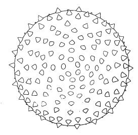
The problem: To improve the aerodynamic stability of spherical balloons used to measure the intensity and direction of atmospheric winds at various elevations. Because standard smooth-surfaced sounding balloons are aerodynamically unstable, they ascend erratically, even in gentle winds, and are therefore difficult to track.
