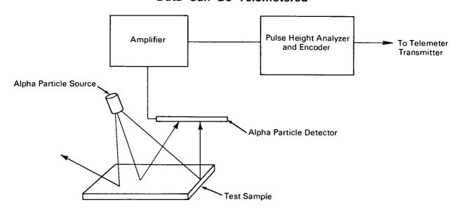
**The problem:** Devising a lightweight instrument for nondestructive chemical analysis of surfaces. The instrument must automatically perform the analysis and provide the resultant data in the form of electronic signals which can be transmitted to remote sites. Such an instrument was particularly required for chemical analysis of lunar and planetary constituents and transmission of the data via telemetry to receiving stations on the earth.
