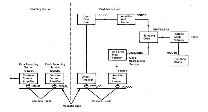
**The problem:** To design a reliable, precision PCM (pulse code modulated) magnetic tape recording and reproducing system that achieves a high packing density on the tape and provides a symmetrical reproduction of the recorded signal.
